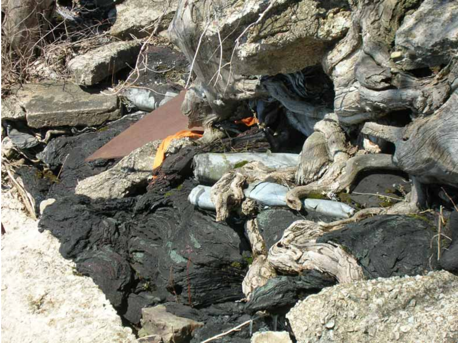
Western Bank of Site on Presque Isle Bay – Tar Expression and Asbestos Paper Rolls
